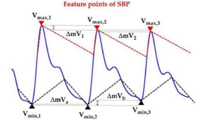
**Fig. 1**: Peak and valley detection algorithm for pressure pulse wave (PPW) signals.<sup>21</sup>
